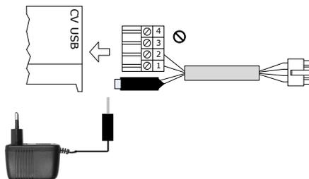
X 1 (8-core) connection for CP 35 plug on the wire harness
