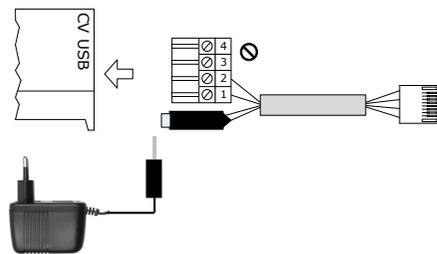
RJ 45 connection for RJ 45 plug at the wire harness
